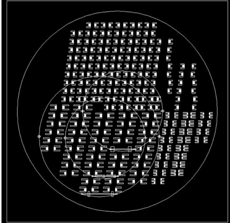
Fig. 4.4 The 6-inch photo mask with IDT patterns used in this work.
