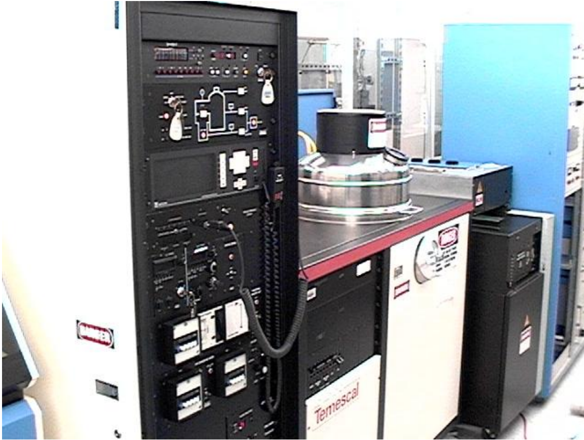
Fig. 4.6 The E-beam evaporation equipment BJD1800 in SIMM clean room
